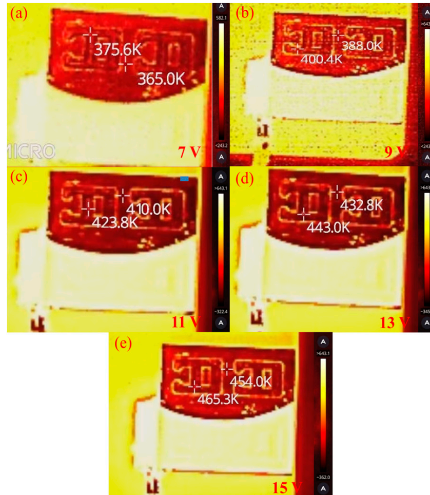
Figure 15. Results of infrared thermometers at different voltages: (a) 7 V, (b) 9 V, (c) 11 V, (d) 13 V, (e) 15 V.
