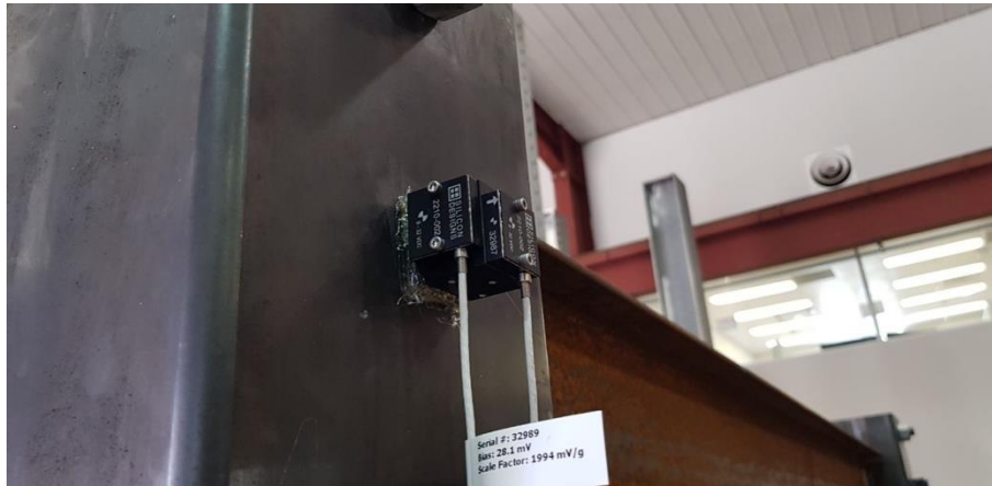
Figure 6. Accelerometers mounted at the top of module's column.
