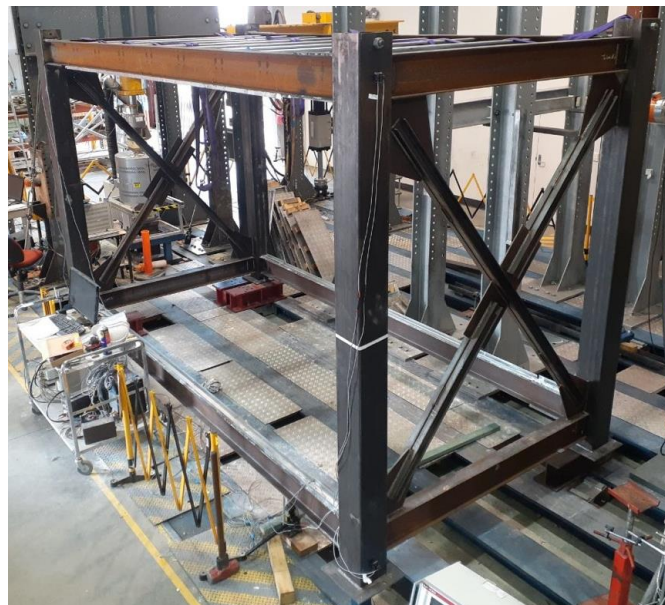
Figure 2. Fabricated module fixed to the strong floor.
