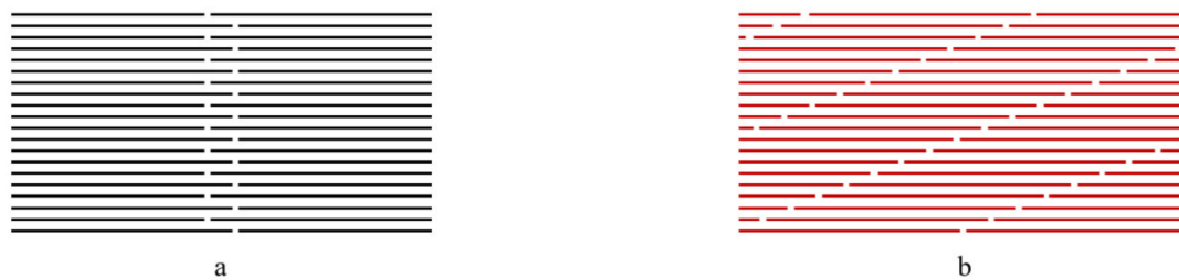
Figure 3. The diagram of (a) vertical and (b) stair-like splicing structures of the laminated composites.
