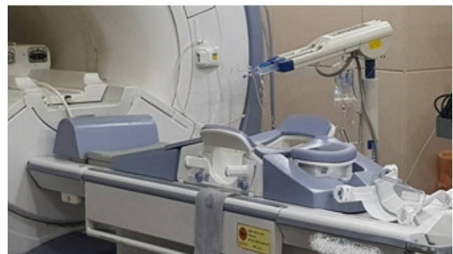
Fig. 1. Patient position assist device for breast MRI, including an 8-channel breast coil ® (GE Healthcare, USA). MRI: magnetic resonance imaging.
