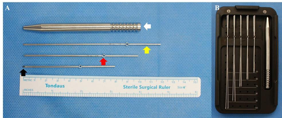
**Fig. 2** Ring pin set (Jeil Medical, Seoul, Korea). **(A)** It consists of three parts: the proximal tail (yellow arrow) for securing the grip for the power drill, the ring (red arrow) for the passage of the cerclage wire, and the sharp distal end for intramedullary insertion into the ulna (black arrow). A snapper (white arrow) is used for further advancement of the ring pin and removal of the proximal tail (yellow arrow). **(B)** Ring pins are provided in lengths from 50 mm to 100 mm
