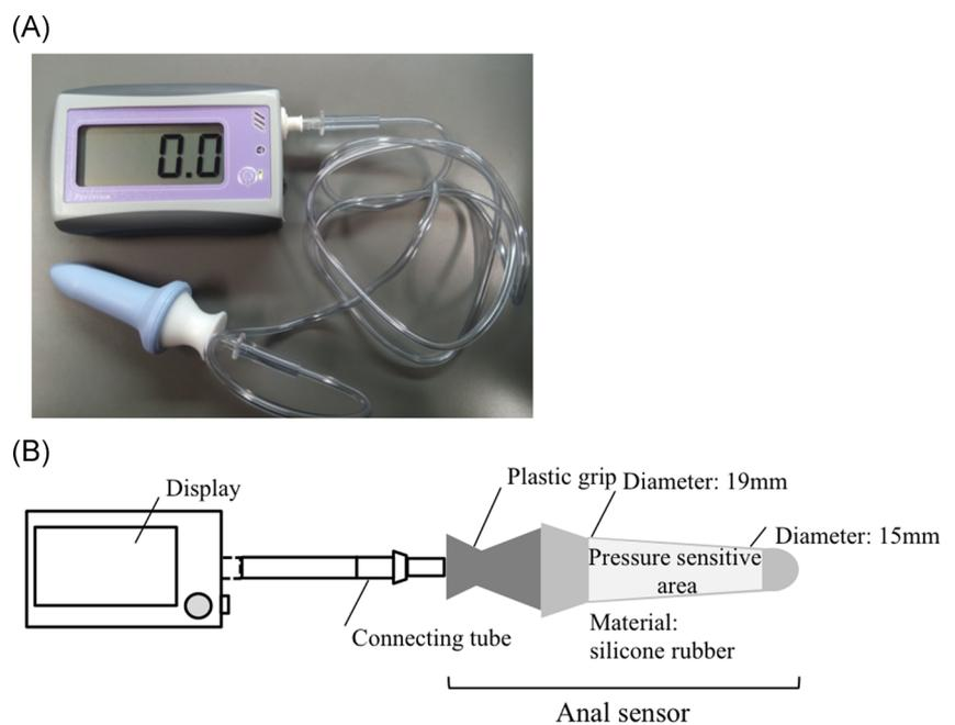
**FIGURE 1** A, Peritron cat 9300A (Laborie, Canada). B, Materials for the Peritron 9300A. Anorectal pressure was assessed as pelvic floor muscle function. During voluntary contractions of the pelvic floor muscle, signal pressure measurements from the pressure-sensitive area of the anal sensor were interpreted by a microprocessor, and a numerical value was displayed in cm H<sub>2</sub>O
