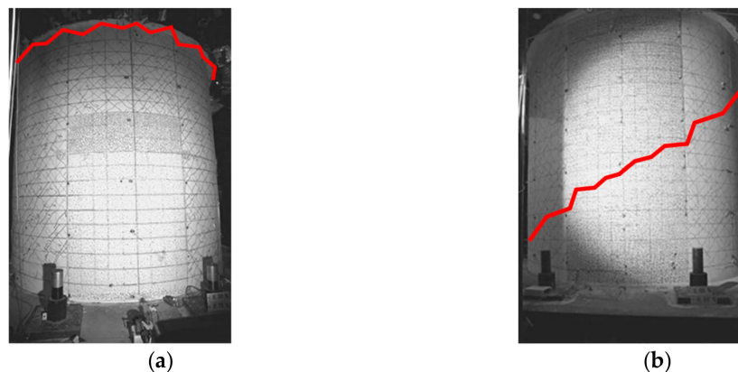
Figure 12. Failure modes of RC containment vessel (RCCV) RCCV#1 and RCCV #2. (a) Sliding shear failure of RCCV #1; (b) Web shear failure of RCCV #2.
