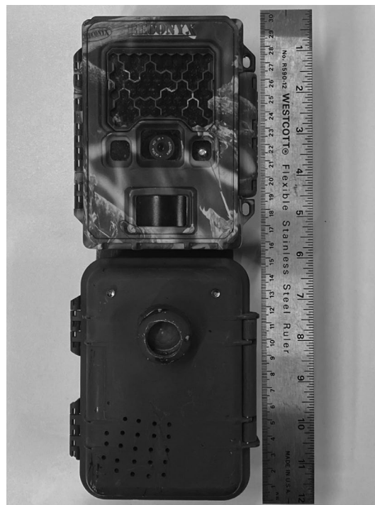
FIGURE 1 A standard camera trap with an “Attention caller device” (ACD). The camera and ACD were deployed together, and both triggered by motion. When activated, the ACD emitted light and sound to attract the attention of a puma, resulting in direct images of the puma's face. Camera traps and ACDs were deployed 2017–2020 in northwest Wyoming
