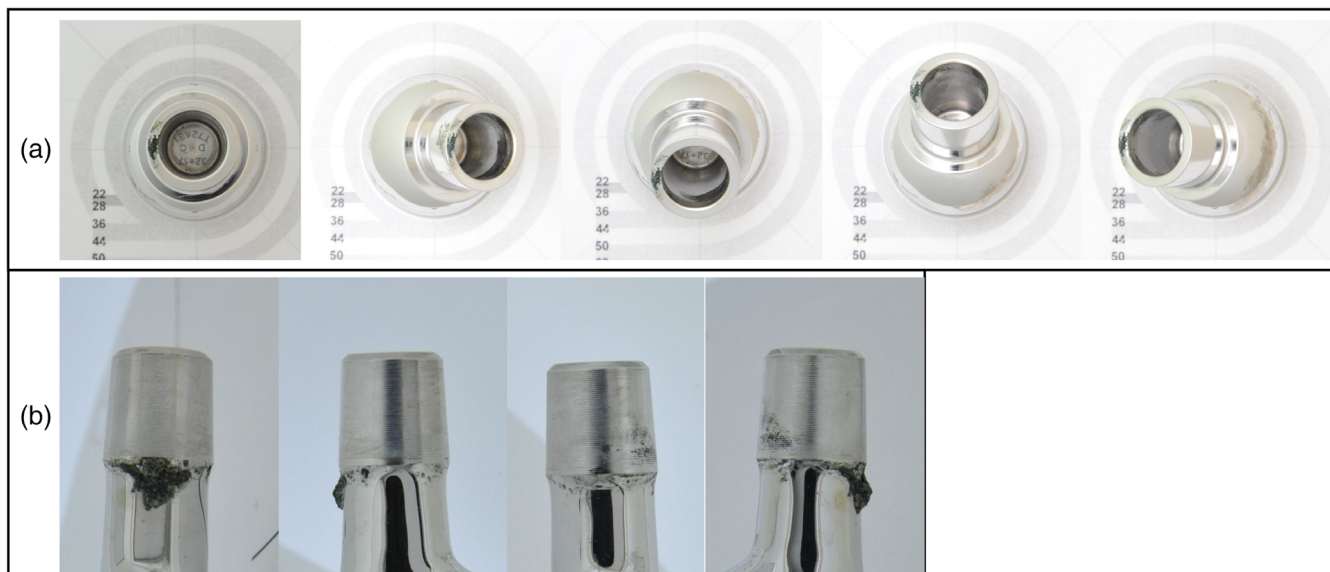
FIGURE 1 Visual scoring method. Example images of the five standardized positions of the femoral head taper (a) and four standardized positions of the femoral stem trunnion (b) used for visual scoring 11
