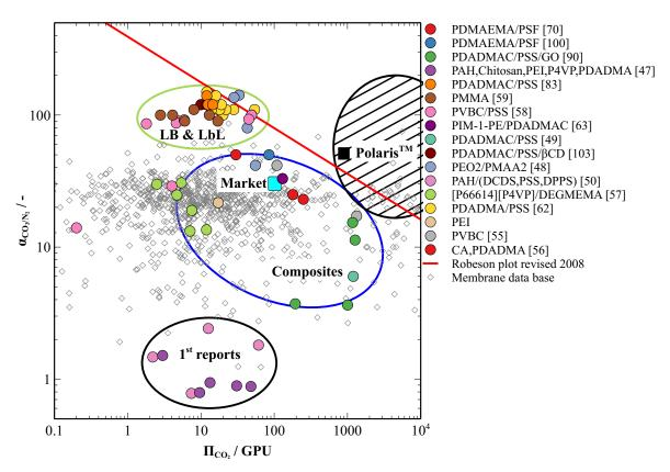
**Figure 9.** Comparison of PE-based membranes for  $CO_2$  separation from flue gas on the R-M plot where the value indicated with the cyan square represents the market standard for  $CO_2$  removal from natural gas and the value indicated with the black square represents the best performing membrane for  $CO_2$ capture available on the market. The striped area suggests the desirable separation performance of  $CO_2$  selective membranes for efficient capture from flue gas.
