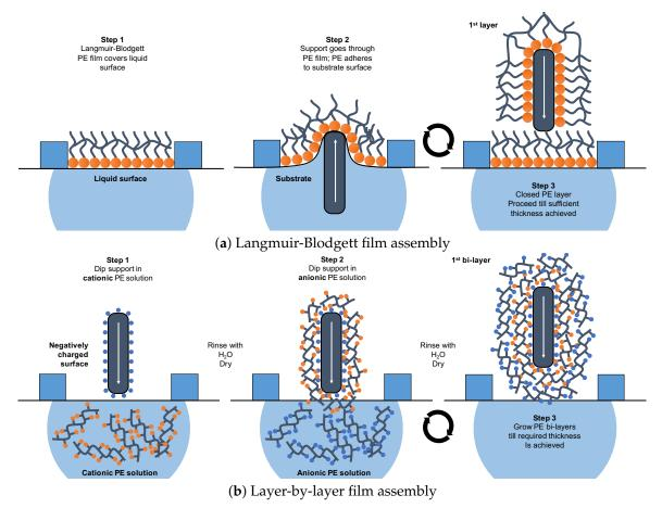
Figure 7. Physical layer deposition of polyelectrolyte films based on ionic interactions.
