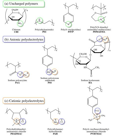
**Figure 4.** Chemical structures of polymers and polyelectrolytes used as precursors for post-synthetic material modification in membrane-based CO<sub>2</sub> capture.
