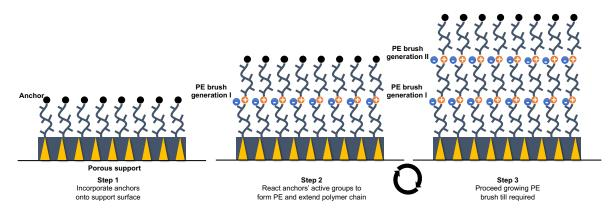
Figure 8. Film membranes Chemical layer deposition via grafting method.
