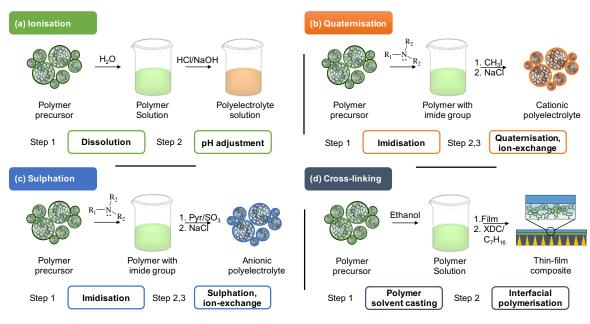
**Figure 5.** Major approaches for post-synthetic modification of polymer to produce 'top-down' polyelectrolytes include (**a**) ionisation, (**b**) quaternisation, (**c**) sulphation, (**d**) cross-linking. XDC abbreviates p-Xylylene dichloride.
