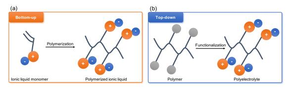
**Figure 2.** Crucial difference between polymerised ionic liquids (PILs) (**a**) and post-synthetic or 'top-down' modification of polyelectrolytes (**b**) stems from chemical origin of polymer chain bearing the ionic charges. In PILs it forms by polymerisation of ionic monomers, and in 'top-down' polyelectrolytes it is already present in parent material.
