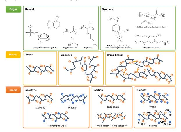
Figure 3. Origin, matrix, and charge in polyelectrolytes.
