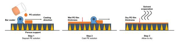
Figure 6. Physical layer deposition via solvent-casting method.
