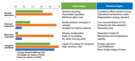
**Figure 1.** Comparison of existing  $CO_2$  capture technologies based on the energy demand for achieving certain volumetric ratio of  $CO_2$  in product stream and respective  $CO_2$  content in feed stream presented alongside the most common advantages and disadvantages of each process. The numerical data is collected across several publications and presented as reported [4–9].
