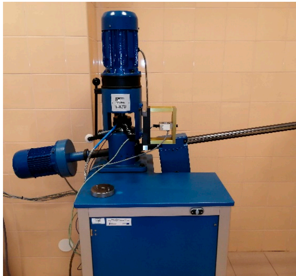
Figure 1. The four-ball machine T-02U used to determine the lubricity tests.
