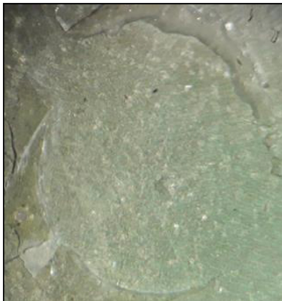
Fig. 2 (Original magnification \times 20 ) Resin cement shows adhesive failure.
