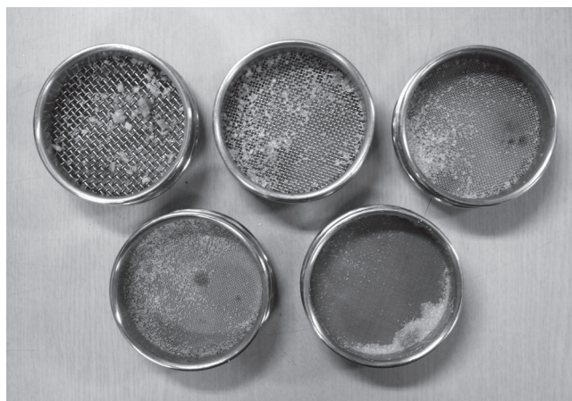
Figure 1. Internationally accepted standard sieve system.
