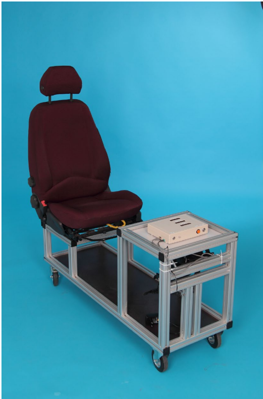
Fig. 1 The driving simulator with an adjustable seat and the electronics. The trigger and a green lamp are orientated towards the observer
