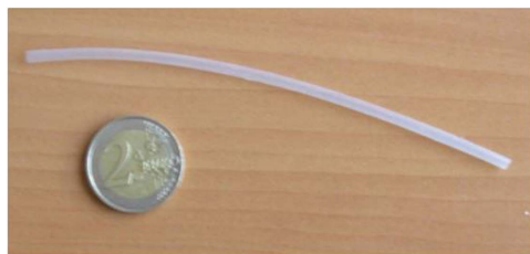
Figure 6. Extruded tube of P(VDF-TrFE-CTFE) with 15%wt DEHP.
