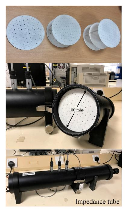
Figure 3. 3D printed samples of MPPs and the setup of the acoustic absorption test.
