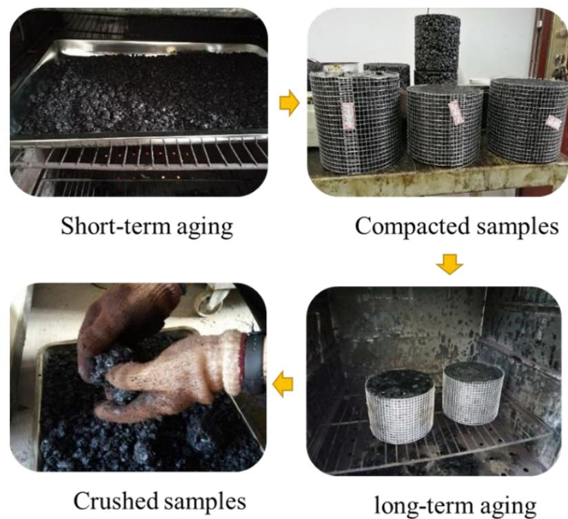
**Figure 4.** The process illustrating RAP production.
