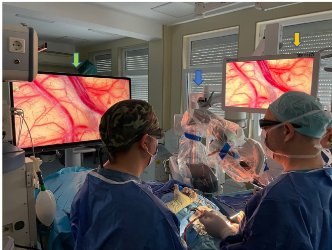
Fig. 6. Intraoperative photograph of the setup during a cranial operation. The Robotic Digital Microscope /marked with blue arrow/ is positioned to the right of the patient, next to the right hand of the neurosurgeon and next to the operating nurse. In this setup the main screen /yellow arrow/ of the RDM is used by the assistant and the additional wider screen /green arrow/, placed at the foot of the operating table, is used by the neurosurgeon. Notice the straight comfortable position of both neurosurgeons and the unobstructed line of view between them and the screens of the RDM. (For interpretation of the references to colour in this figure legend, the reader is referred to the Web version of this article.)
