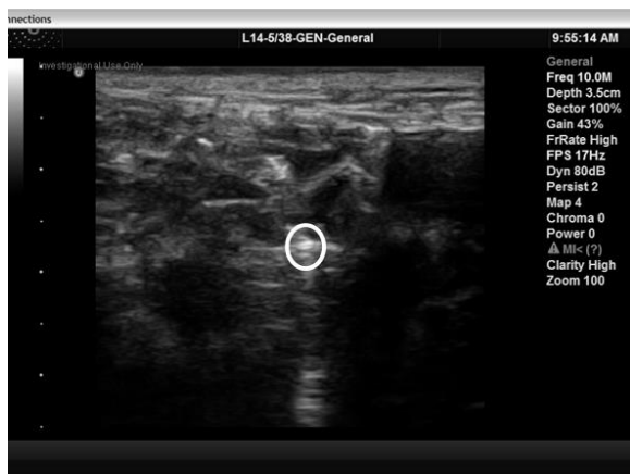
FIGURE 7. Ultrasound B-Mode image of a typical thermal lesion post HIFU exposure. The lesion is visible as a hyperechoic region which coincides with the location of the HIFU focal point in the ROI (ellipse).
