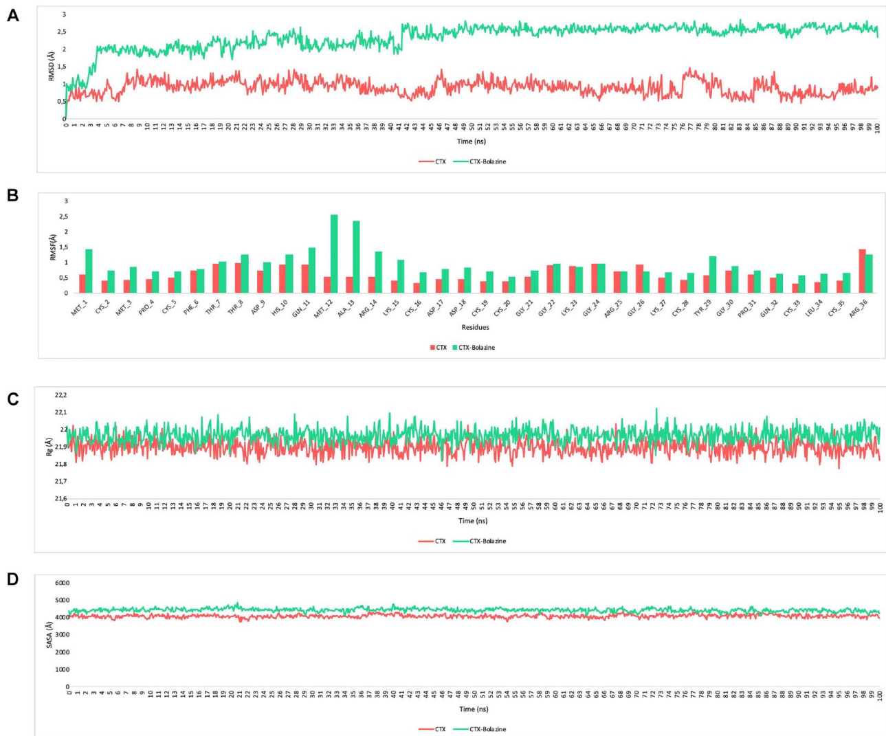
Figure 4. Plots of structural fluctuations of CTX alone (red) and CTX–bolazine complexes (green) over 100 ns molecular dynamics simulation. (A) The RMSD values in Angstroms (Å) over simulation time. (B) The RMSF values in Angstroms (Å) along the residue positions. (C) The Rg values in Angstroms (Å) through the simulation time (ns). (D) The SASA values respectively, in Angstroms (Å) through the simulation time (ns).
