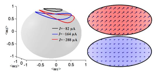
Figure 3 | Micromagnetic simulations for sample 1. Left. Trajectories of the average magnetization vector on the unit sphere as computed from micromagnetic simulations (I = -82, -164 and  $-288 \mu$ A). Right: example of two snapshots of the spatial distribution of the magnetization indicating the uniform dynamics (the color means the x-component of the magnetization blue negative, red positive).
