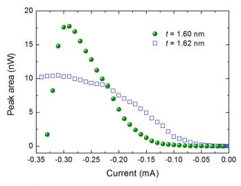
**Figure 2** | **Power of STNO samples.** Integrated power of fundamental signals at zero applied magnetic field as a function of *I*. Olive circles are for 1.60 nm sample and blue squares for 1.62 nm sample.
