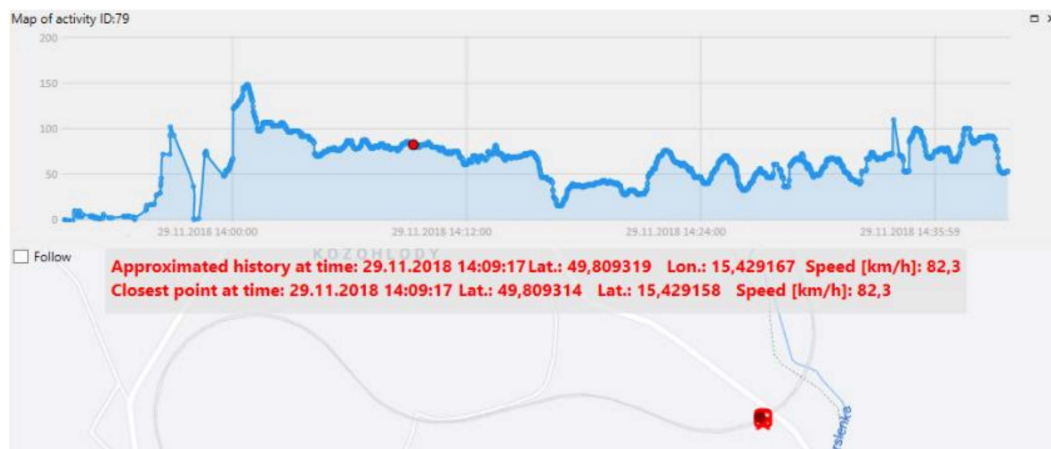
Figure 22. The speed profile of the train and its map location at selected time instant.
