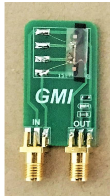
Figure 7. The test module of the amorphous wire alloy magnetic sensor impedance. The diode detector circuit consists of a capacitor, a resistor and a diode.
