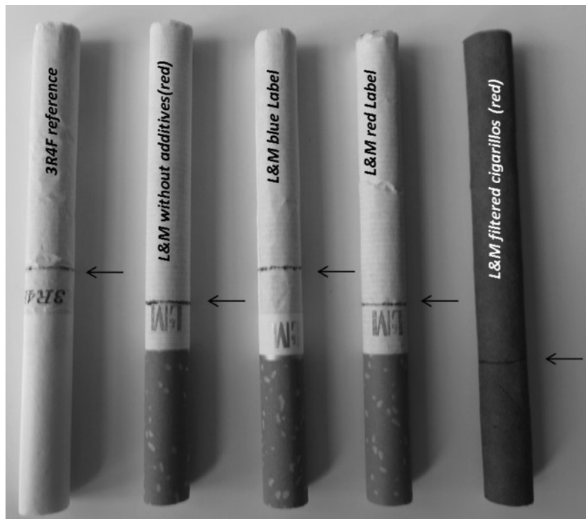
Figure 2. Examined tobacco products: The sample size was 20 of each tobacco product. The arrows mark a distance of 8 mm from the tipping paper. The cigarettes and cigarillos were all smoked down to this mark.
