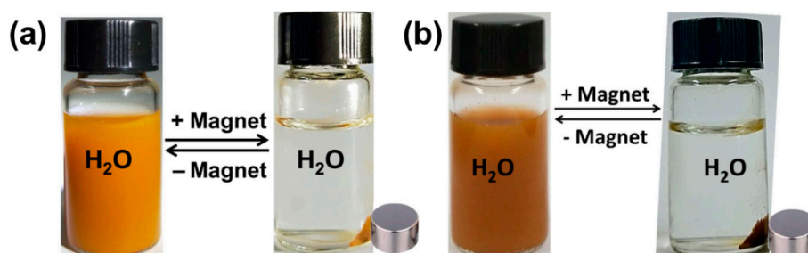
Figure 5. The dispersion-collection process of (a) \text{Fe}_3\text{O}_4@1 and (b) \text{Fe}_3\text{O}_4@2 .
