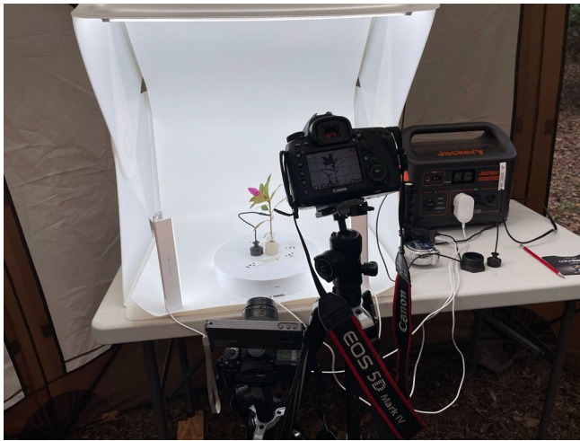
FIGURE 1 The battery-powered Foldio set-up with our two cameras on tripods set at different heights and a supplementary LED light on the hot shoe of the lower camera inside our pop-up work shelter. The scene demonstrates the use of an alligator clip to support the positioning of a branch in the center of the turntable, with the end of the branch anchored in a water-containing Eppendorf tube surrounded by modeling clay. The two 10-cm scale bars are attached to the turntable with double-sided tape.
