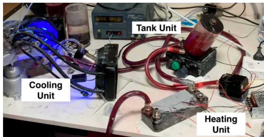
Figure 17. Current prototype of thermochromic heater-cooler system.
