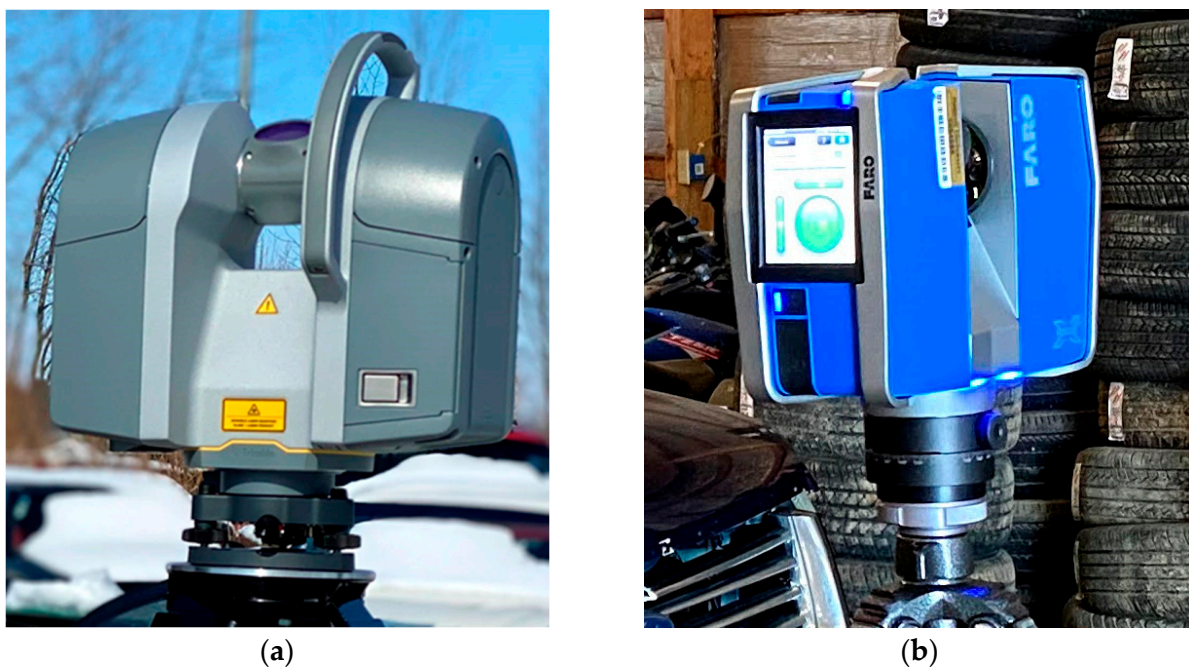
Figure 3. Terrestrial Laser Scanning (TLS) equipment: (a) Trimble TX8b Laser Scanner; (b) FARO Focus 3D X330 Laser Scanner.
