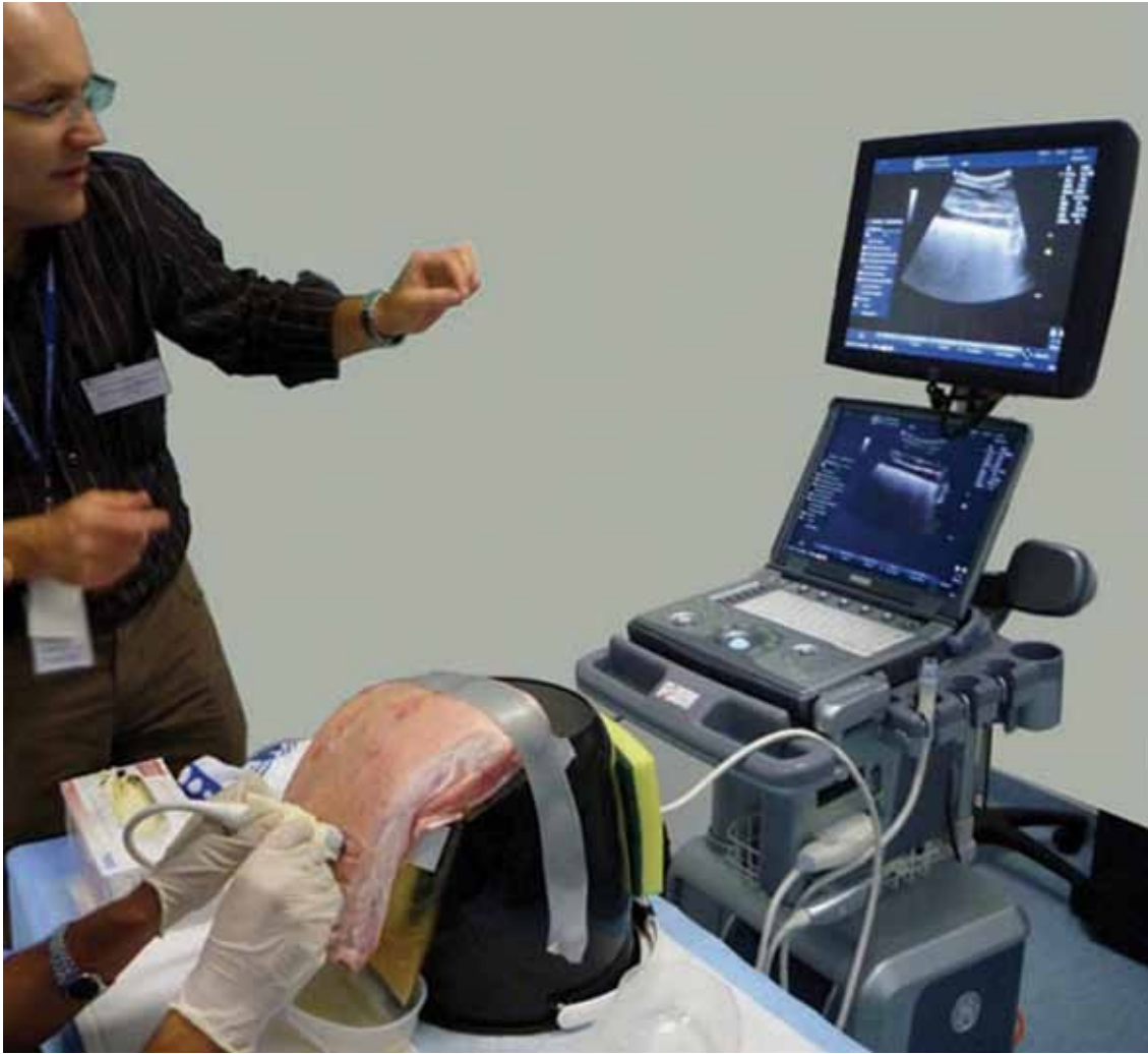
Figure 4: The phantom in use; note the operator, transducer, phantom and ultrasound screen are all in line. In this case a small amount of psyllium husk has been added to the fluid to create the appearance of empyema.
