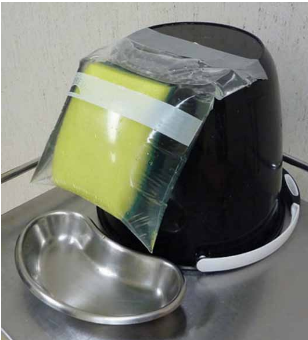
Figure 2: The bucket creates the framework for the phantom. The plastic bag filled with water and a sponge simulates the pleura, effusion and lung.
