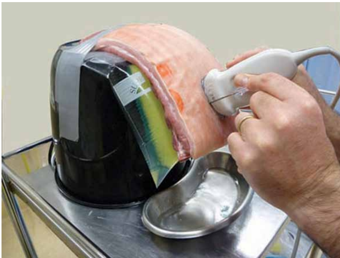
Figure 3: The pork rib is placed over the bag and attached to the bucket; this simulates the human chest wall. Ultrasound gel may be required between the rib cage and the bag. Note: An ultrasound probe cover and gloves are recommended but were excluded from these photographs for visual simplicity.
