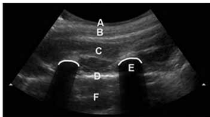
Figure 8: Thoracic phantom using pork ribs and sponge with curvilinear probe.
