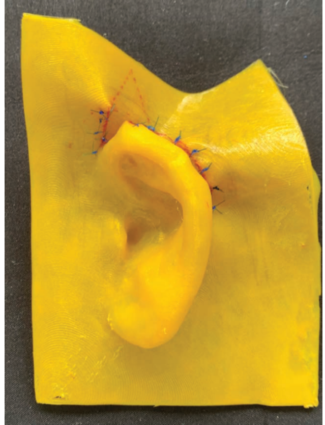
Fig. 2. The 3D model after simulated cat's-ear flap surgery. The model could be bent like a human ear. Moreover, the flap could be designed on the model, after which the material could be incised and sutured like human skin during an operation. Another model was subjected to simulated square flap surgery, allowing comparison of esthetic outcomes between the 2 methods for this particular case.
