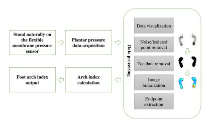
Figure 1. The framework of the proposed algorithm.
