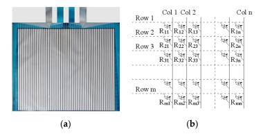
Figure 3. Flexible membrane pressure sensor. (a) Flexible membrane pressure sensor. (b) Equivalent circuit of sensing points.
