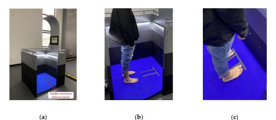
**Figure 8.** Prototype of foot arch index measurement. (**a**) is the designed prototype, and (**b**) and (**c**) show the correct test position.
