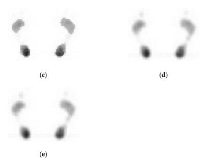
**Figure 4.** (a) shows the definition of the 8-neighborhood correlation pixel and (b) is the original plantar pressure image generated by the sensor data and the result after using the 8-neighborhood correlation pixel method. (c) is the result of median filtering, (d) is the result of Gaussian filtering and (e) is the result of mean filtering.
