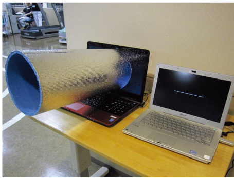
Fig. 1. Assessment of subjective visual vertical These two computers were linked with an USB cable so that the image displayed on the computer controlling the SVV was also displayed on the computer screen that the subjects watched. a cylindrical tube was placed in such a manner that the vertical portion of the screen frame could not provide clues to verticality.
