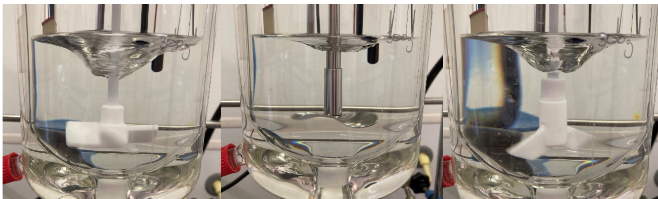
Figure 8. Vortex produced by different stirrer types at 300 rpm.
