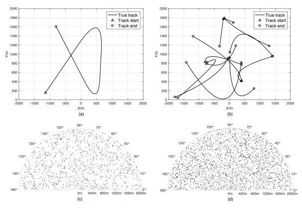
**Figure 1.** True trajectories of targets and clutters. (**a**) Target trajectories in Scenarios 1 and 2. (**b**) Target trajectories in Scenarios 3 and 4. (**c**) Clutter distribution in Scenarios 1 and 2. (**d**) Clutter distribution in Scenarios 3 and 4.
