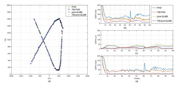
**Figure 4.** Result comparisons in Scenario 1. (**a**) Position estimations of the original random finite set (RFS)-based filters and the time-matching filters in one trial. (**b**) Optimal subpattern assignment metric (OSPA) errors. (**c**) Location components of OSPA. (**d**) Cardinality components of OSPA. PHD, probability hypothesis density; GLMB, generalized labeled multi-Bernoulli filter.
