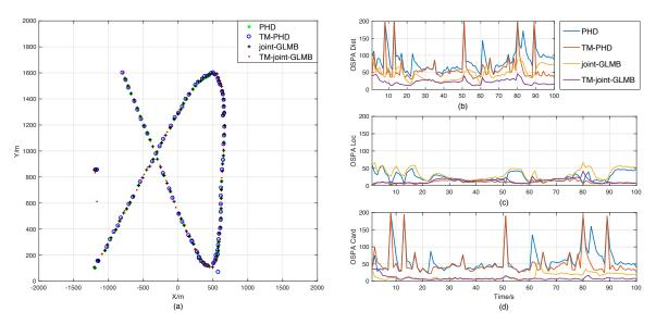
**Figure 5.** Result comparisons in Scenario 2. (**a**) Position estimations of the original RFS-based filters and the time-matching filters in one trial. (**b**) OSPA errors. (**c**) Location components of OSPA. (**d**) Cardinality components of OSPA.
