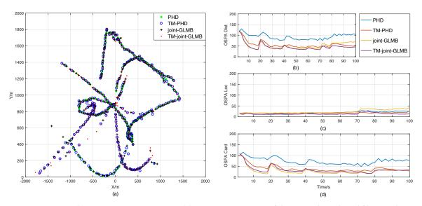
**Figure 6.** Result comparisons in Scenario 3. (a) Position estimations of the original RFS-based filters and the time-matching filters in one trial. (b) OSPA errors. (c) Location components of OSPA. (d) Cardinality components of OSPA.
