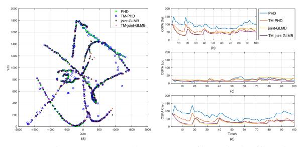
**Figure 7.** Result comparisons in Scenario 4. (**a**) Position estimations of the original RFS-based filters and the time-matching filters in one trial. (**b**) OSPA errors. (**c**) Location components of OSPA. (**d**) Cardinality components of OSPA.
