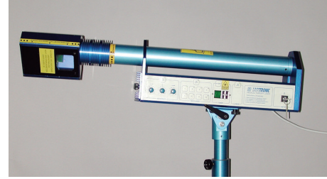
FIGURE 2: Lasotronic Laser device: the device can be adjusted in height, and the laser head can be tilted and rotated to reach the correct position of the laser beam. The turning knobs on the left serve to adjust focus and irradiation patterns. The key on the right is the main power switch.
