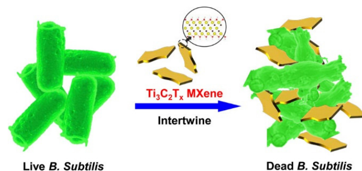
Figure 11. Schematic depiction of antibacterial activity of Ti 3 C 2 T x MXene [3].
