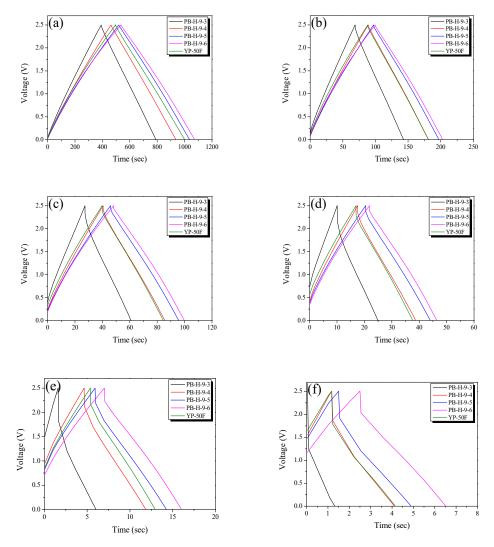
**Figure 6.** Charge–discharge curves of bamboo-derived activated carbon materials as a function of steam activation conditions obtained at (a) 0.1, (b) 0.5, (c) 1.0, (d) 2, (e) 5.0, and (f) 10.0 mV/s.
