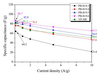
Figure 7. Specific capacitance of PB-AC as a function of discharge current density.
