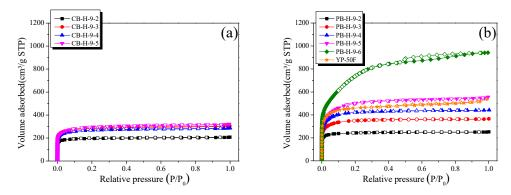
Figure 1. N<sub>2</sub>/77 K isotherm adsorption–desorption curves of (a) CB-AC; (b) PB-AC.
