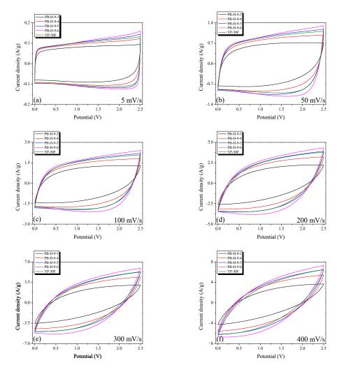
**Figure 8.** Cycle voltammograms of the bamboo-derived activated carbon samples at various scan rates: (a) 5, (b) 50, (c) 100, (d) 200, (e) 300, and (f) 400 mV/s.
