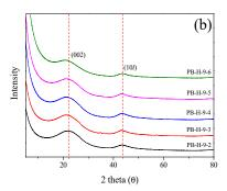
**Figure 3.** XRD patterns of bamboo-derived activated carbon as a function of various steam activation conditions: (a) CB-AC and (b) PB-AC.
