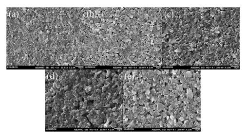
**Figure 5.** SEM images of the activated carbon electrodes (a) PB-H-9-3, (b) PB-H-9-4, (c) PB-H-9-5, (d) PB-H-9-6, and (e) YP-50F.
