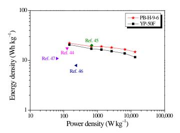
**Figure 11.** Ragone plot of the bamboo-derived activated carbon device compared with data in other literature studies.
