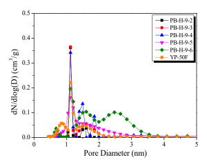
**Figure 2.** Pore size distributions obtained using the NLDFT method of the bamboo-derived activated carbon as a function of steam activation conditions.
