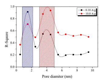
**Figure 10.** Correlation between the specific capacitance of the PB-AC samples and pore volume. The *x*-axis shows the average PSD plotted as pore volume according to pore diameter in 1 nm units using the average value of each PSD.
