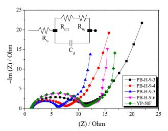
**Figure 9.** Nyquist plots of bamboo-derived activated carbon materials obtained using different steam activation conditions and its equivalent circuit is shown in inset.
