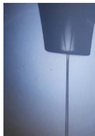
Figure 15 Photograph of a 100 \mu\text{m} -diameter round liquid jet with quartz glass capillary at a flow speed of 30 \text{m s}^{-1} .
