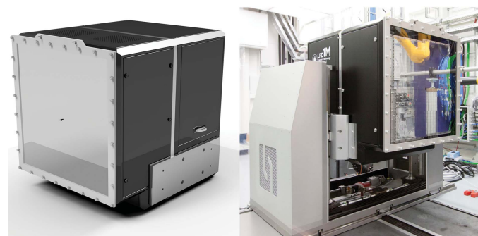
Figure 11 The Large Pixel Detector (left: design, right: as installed inside the FXE hutch) has 1 million pixels, each with 0.5 \times 0.5\text{ mm} size. The detector can store at maximum 510 images sampled with a frequency of 4.5 MHz. Each single-shot image has a dynamic range of about 1 \times 10^5 12 keV photons.
