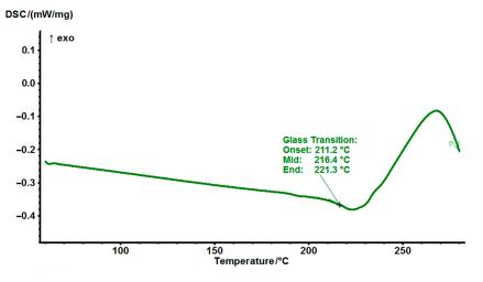
Figure 6. DSC thermograms cured EG513 at a heating rate of 10 °C/min.
