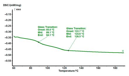
the glass transition temperature of 90  $^{\circ}$ C is characteristic for this resin with other hardeners (Figure 10).
