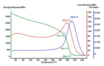
Figure 11. DMA thermogram of EG514.
