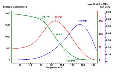
Figure 12. DMA thermogram of EG531.
