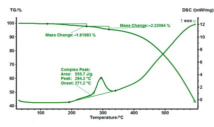
**Figure 4.** STA-thermograms of MPD-TPA-MPD in the air atmosphere at a heating rate of  $10 \,^{\circ}$ C/min.
