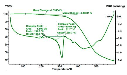
**Figure 3.** STA-thermograms of MPD-TPA-MPD in nitrogen atmosphere at a heating rate of  $10 \,^{\circ}\text{C/min}$ .
