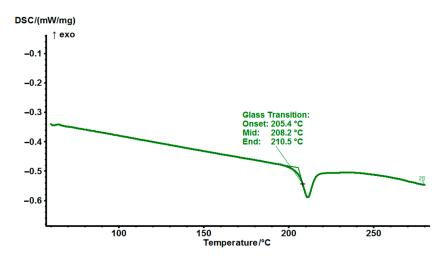
**Figure 8.** DSC thermograms cured EG514 at a heating rate of 10  $^{\circ}$ C/min.
