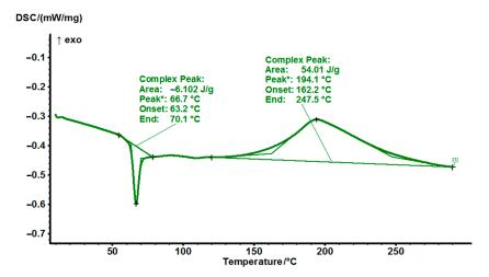
Figure 9. DSC thermograms of non-cured EG531 at a heating rate of 10  $^\circ$ C/min.
