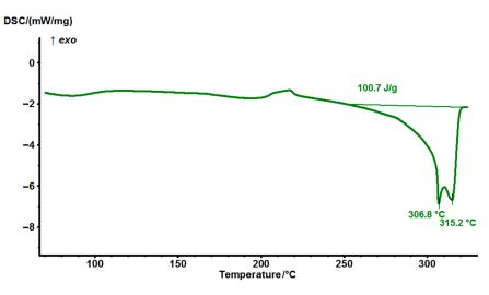
Figure 2. DSC thermograms of MPD–TPA–MPD at a heating rate of 10 °C/min.
