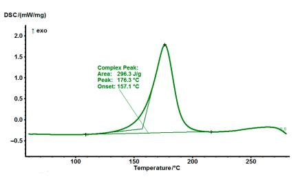
Figure 5. DSC thermograms of non–cured EG513 at a heating rate of 10 °C/min.
