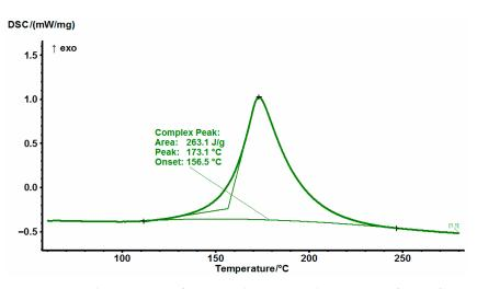
Figure 7. DSC thermograms of non-cured EG514 at a heating rate of 10 °C/min.
