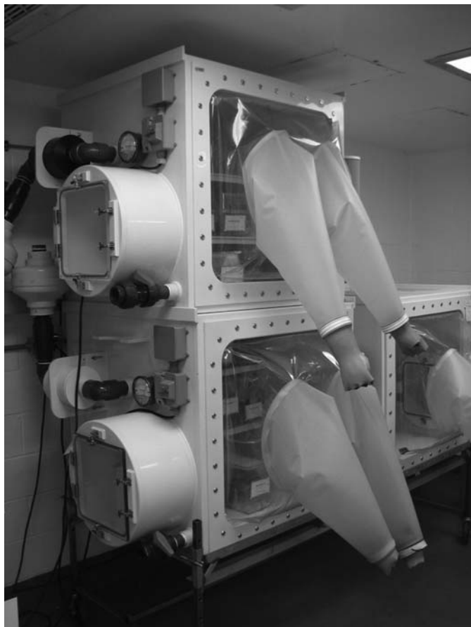
Fig. 26-5 Stacked semi-rigid isolators suitable for rodent quarantine activities.
