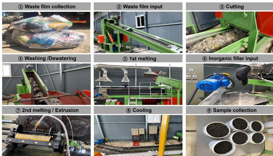
Figure 1. Production processes of recycled plastic film-based aggregates.
