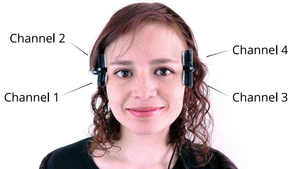
Fig 2. Smile reader. The EMG wearable consists of four channels located as depicted in this figure. Written informed consent was obtained for the publication of this image.
