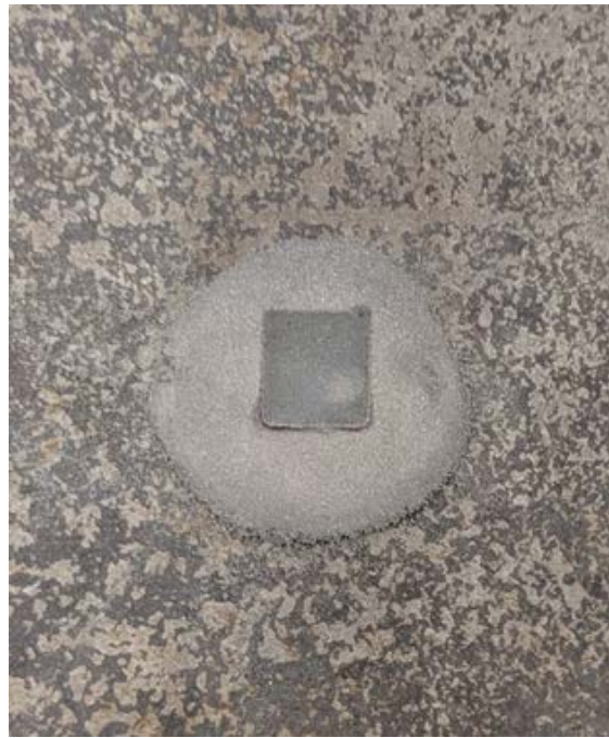
Figure A20. A square shaped HEA printing using selective laser melting technique.
