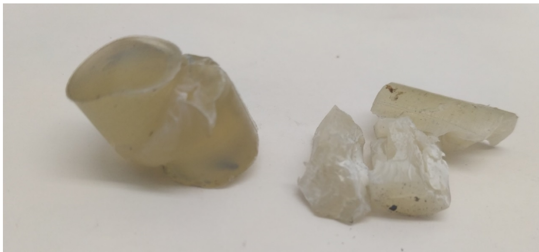
Figure 4. Samples after the compression test. On the left: buckled sample. On the right: fractured sample.
