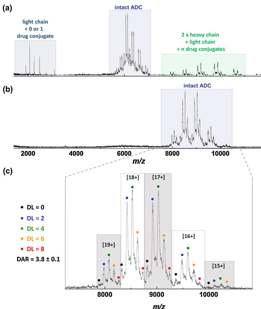
**Fig. 2.** Mass spectra of  $\sim 7 \mu\text{M}$  ADC in 100 mM ammonium acetate (a) and in 100 mM ammonium acetate + 10% TEAA (b) acquired on the Ultima API US mass spectrometer where the sampling cone voltage is held at 200 V. Addition of TEAA shifts the intact protein peaks to a higher  $m/z$  region and preserves non-covalent interactions. (c) Zoom of (b) the intact ADC mass region and assignment of ADC species with different drug load (DL); the average DAR =  $3.8 \pm 0.1$ .
