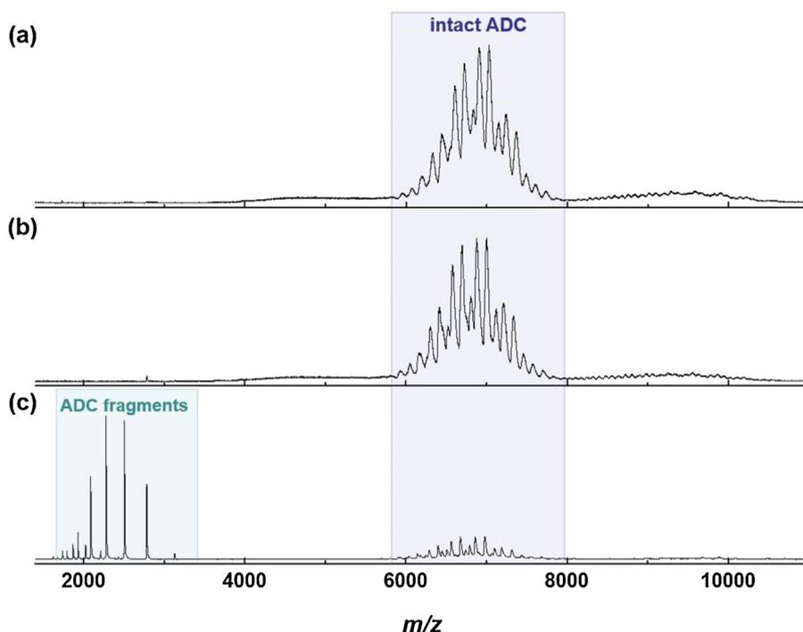
**Fig. 1.** Mass spectra of  $\sim 7$   $\mu$ M ADC acquired on the Q-ToF Ultima API US mass spectrometer at three different acceleration voltages: 50 V (a), 100 V (b) and 200 V (c). Increase of this parameter results in effective in-source salt clean-up during the desolvation process, at the same time leading to dissociation of the non-covalent ADC.
