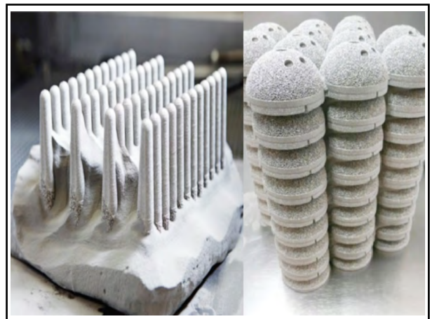
Fig.2: Parts stacked in sintered powder (Courtesy GE Additive). 28
