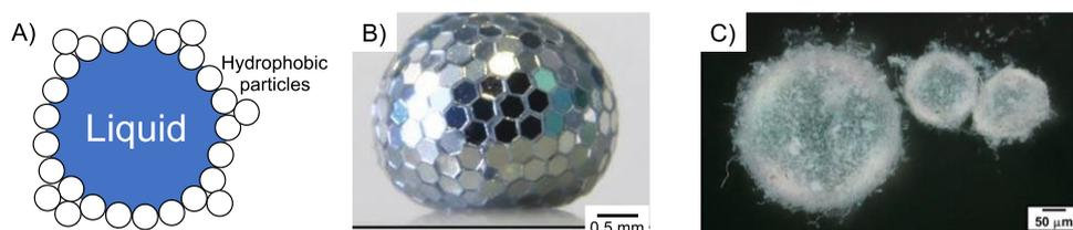
**Figure 3** Schematic figure of liquid marble (A) and microscopic pictures of polyhedral liquid marble (B) and liquid marbles fabricated by aphid (C). The images were adapted with permission from Refs. [20] and [21].
