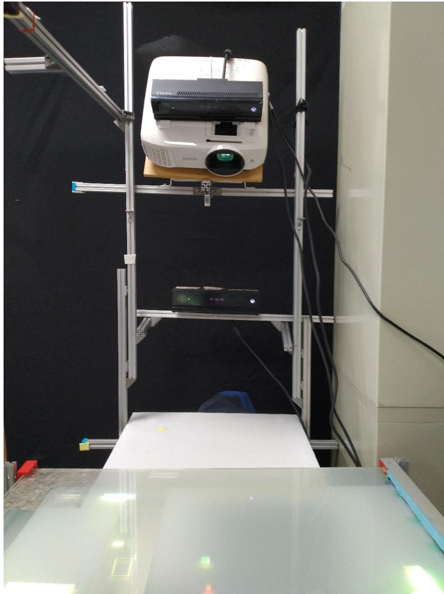
Figure 2. Developed Inspection System Setup.
