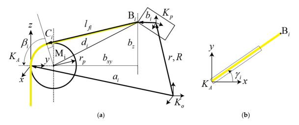
**Figure 10.** Extended pulley kinematics to encounter the pulley geometry into the cable robot kinematics; (a) determination of the point  $C_i$  where the cable exit, and (b) pulley rotation angle  $\gamma_i$  out of the xz-plane.
