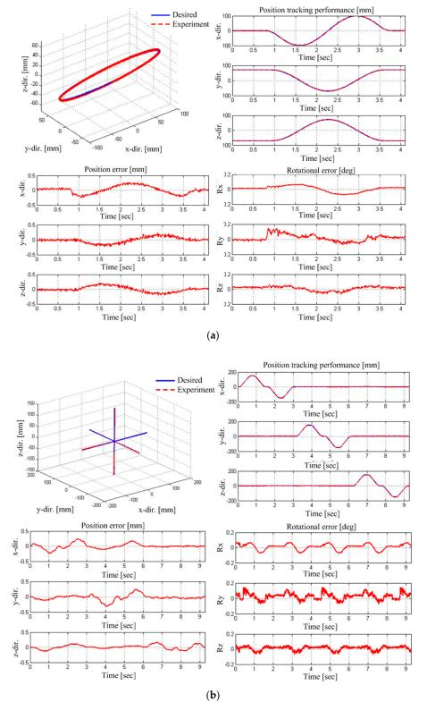
Figure 16. Path accuracy experimental results; (a) circular trajectory and (b) linear trajectory.
