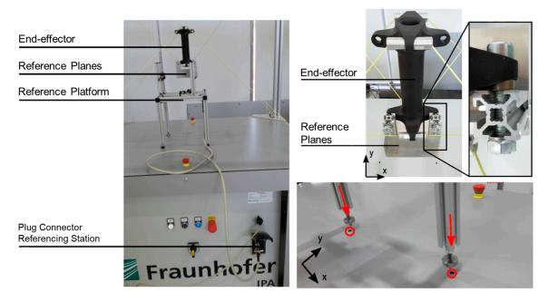
Figure 7. Complete hardware setup to start the referencing procedure.
