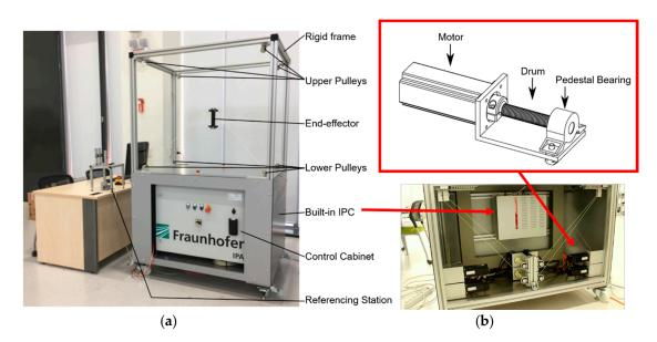
**Figure 2.** The MINI cable robot; (**a**) a photo of the whole MINI cable robot system and (**b**) a winch-motor drawing and actual installation.
