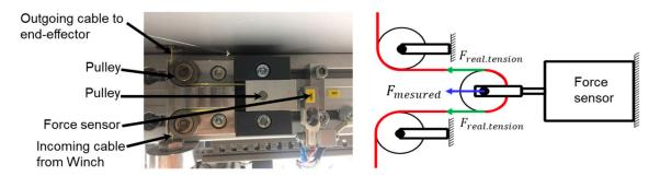
Figure 5. Principles for cable force measurement.
