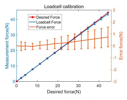
Figure 6. Force sensor calibration results.
