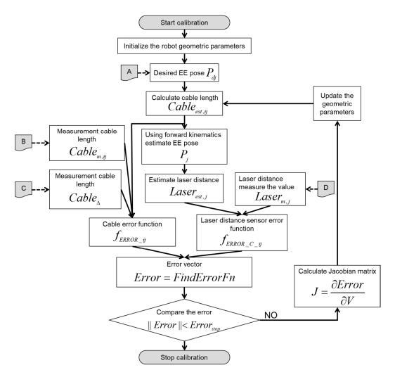
Figure 13. Flowchart of parameter estimation using optimization method in the identification stage.
