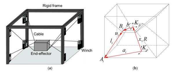
**Figure 1.** Structure schematics of a cable-driven parallel robot with eight-cable configuration; (a) a schematic of the eight-cable-driven parallel robot, (b) kinematic drawing of the cable robot.
