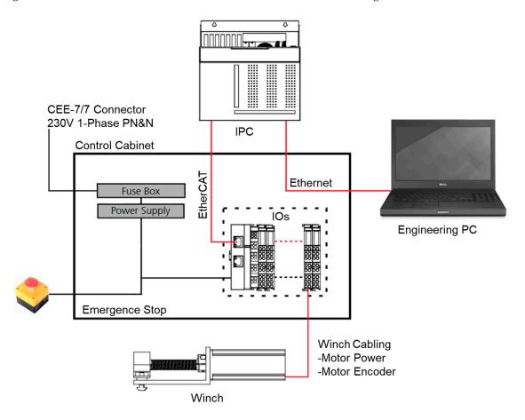
Figure 3. MINI cable robot controller schematics.
