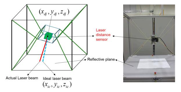
Figure 11. Laser distance sensor setup.
