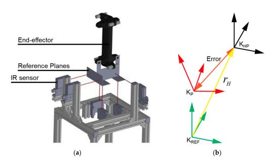
**Figure 8.** Reference platform and coordinate system for the home position reference platform; (a) attachment of the reference planes at the platform, and (b) reference platform coordinate.
