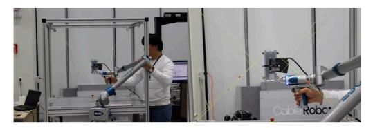
**Figure 14.** A photo-shoot of the actual measurements of the end-effector position using Faro edge ScanArm equipment.
