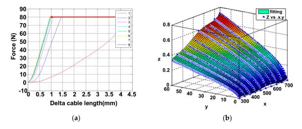
**Figure 9.** Polynomial surface model of the cable elongation as a function of cable length and cable tension measurement; (a) experimental data for different cable lengths and tensions, and (b) surface-fitted model where x is the cable length, y is the cable tension and z is the cable deformation.
