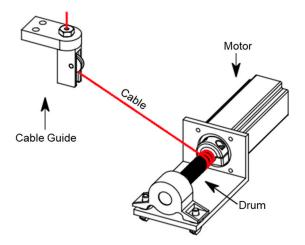
Figure 4. A schematics of the motor-winch component and course of the cable with cable guide pulley.
