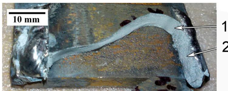
Figure 9. Broken sample #4: (1) core of broken 120Mn3Si2 plate; (2) weld that carried the load in the last stage of failure.
