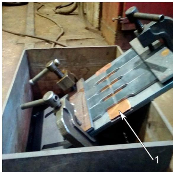
Figure 10. Standard welded samples clamped before welding.
